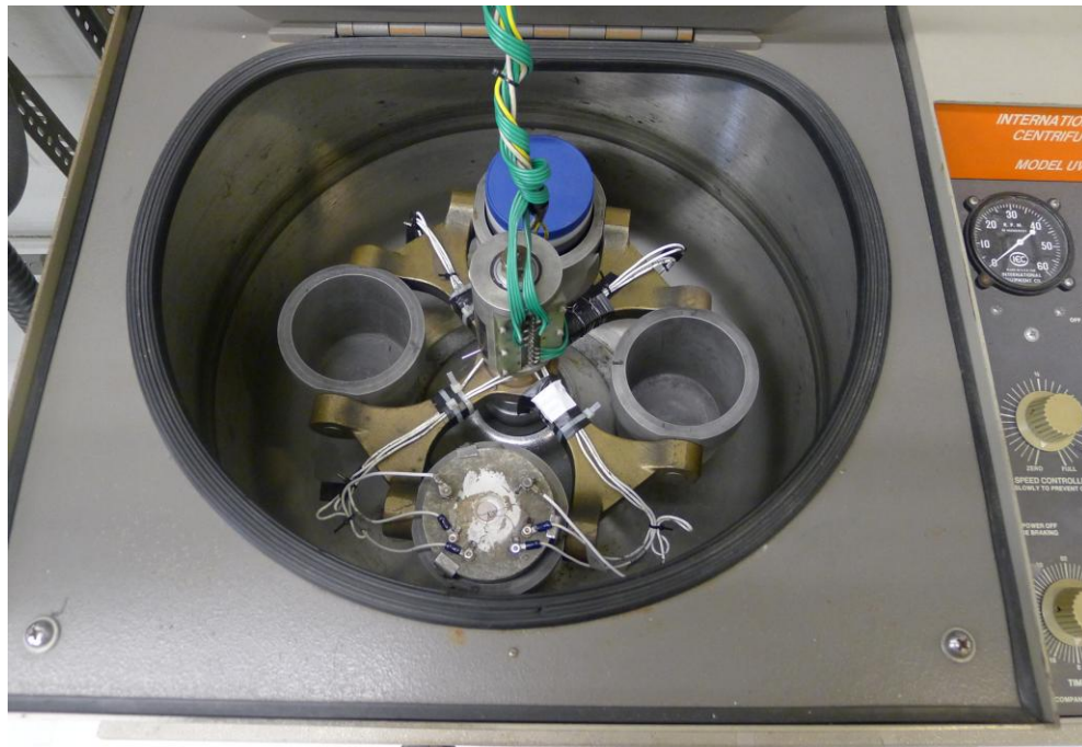
Figure 14. The centrifuge head with its four rotating cups and central slip-ring. The furnace is held by the bottom cup, with three pairs of wires connecting the top of the furnace to the slip-ring. The two pairs of wires connect the two thermocouples of the furnace to the main controller, while the remaining pair provides power to the furnace. A counterbalance filled with sand is held by the top cup.
