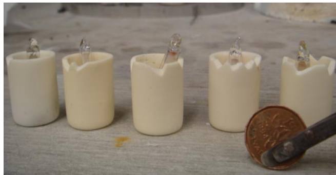
Figure 8. Samples in alumina crucibles before placing them into the furnace. Notches were made on the rims of the crucibles to distinguish the samples from one another.
