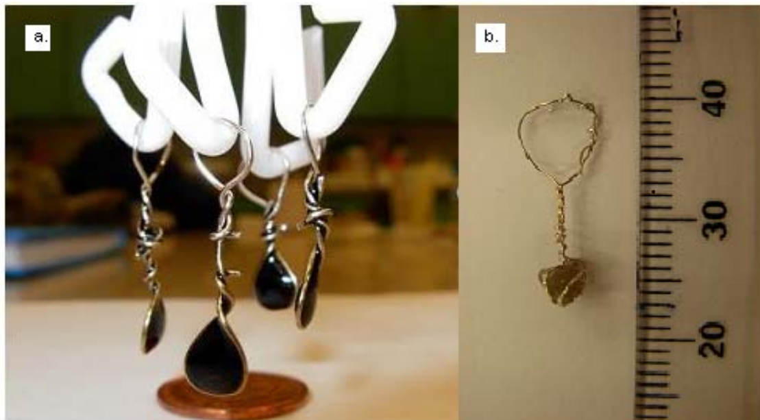
Figure 1: Photo a.) shows a typical assembly used to suspend samples in vertical tube furnace. Photo b.) shows a piece of rhyolite glass used as an alternative to ground material, and wound with Pt/Rh alloy wire.
