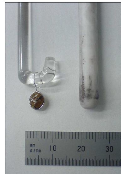
Figure 1. Typical sample + thermocouple assembly.
